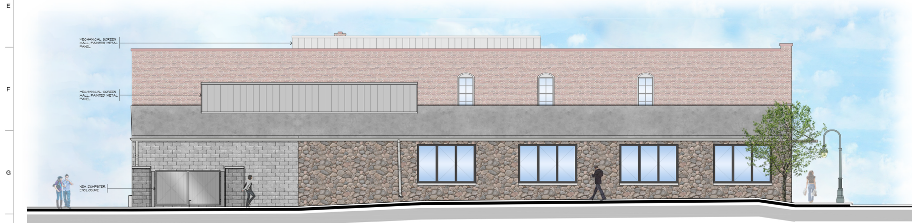
H4 A204 Proposed Side Elevation SCALE: 1/4" = 1'-0"
